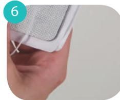
6 Replace electrodes onto their liners and seal them in the re-sealable bag
