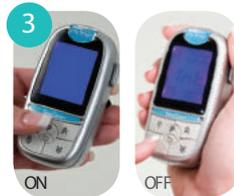
3 Press ON button to check that the unit is working (LCD will be activated) then switch OFF
